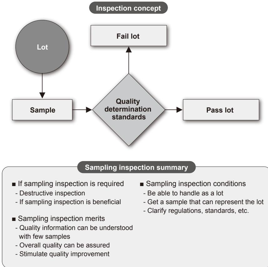
focuses on the quantity of defective items and number of defects, while "measurement-type sampling inspection" deals with the characteristics of measured values.
