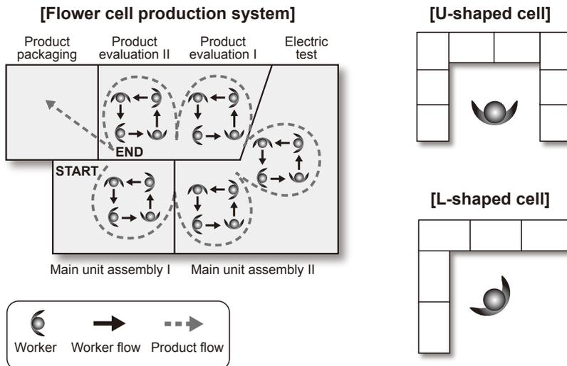
●Figure 8-6 Comparison of Conveyor Production System and Cell Production System
