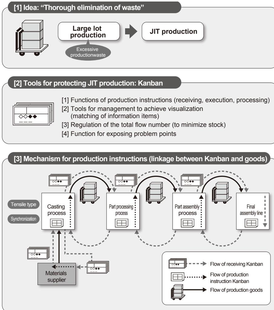
The third point is the “Creation of a mechanism for production instructions” that links Kanban with the actual goods.
