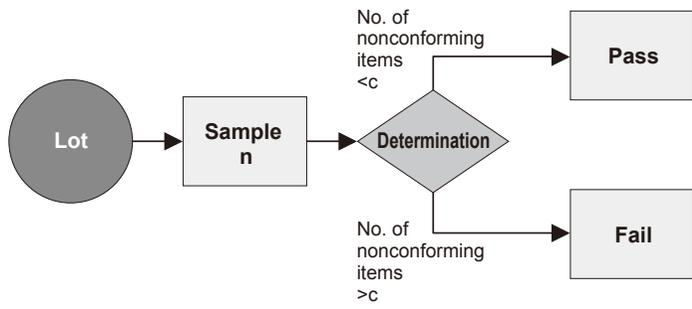
The concept above is called the sampling inspection method, and abbreviated to (n,c).
