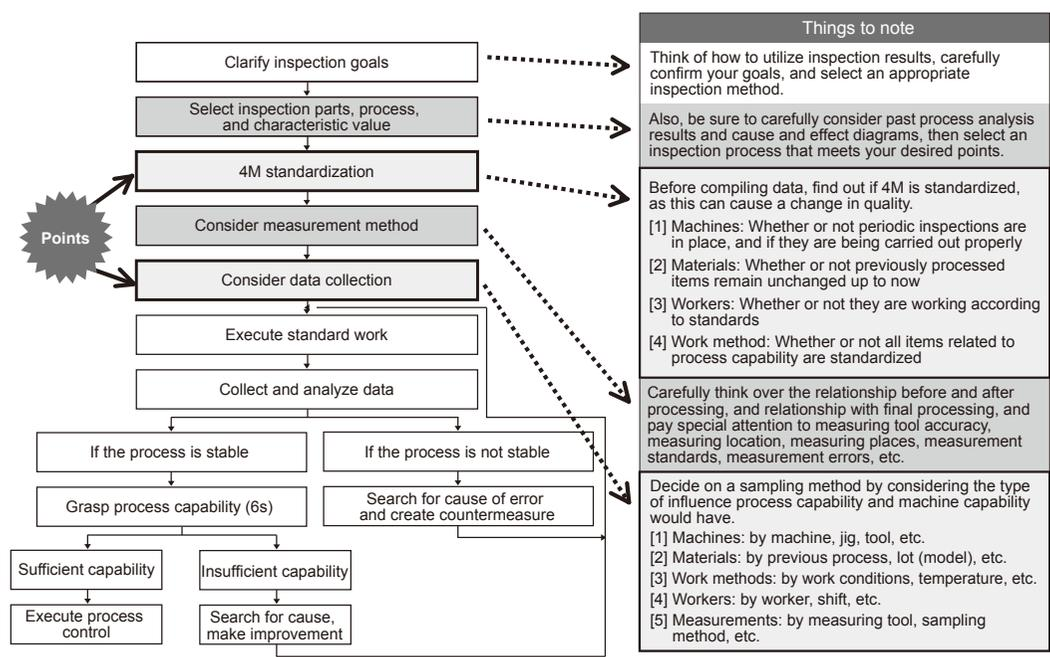
●Figure 5-16 Ways to Determine a Process Capability Index
